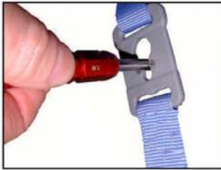
Sling Clip Gauge ST331
