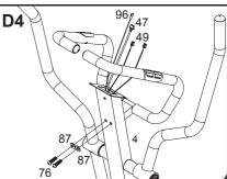
Connect the wires as shown in Figure E1. Connect the Upper Computer Cable (47) to the Computer Connecting Cable (67). Connect the Hand Pulse Cables (49) to the Pulse Connecting Cables (65). Push the cables down into the Upright as you bring the Computer down to attach it. Attach the Computer (23) to the top of the Upright (4), using four M5 X 10mm Dome Bolts (93).
