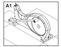
Place a Styrofoam block from the box under the rear of the Main Frame (1). Remove the protective cover from the rear of the Main Frame (1). Attach the Rear Stabilizer (13) to the Main Frame using the preassembled Washers (87) and Bolts (68). Repeat the procedure for the Front Stabilizer (2).
