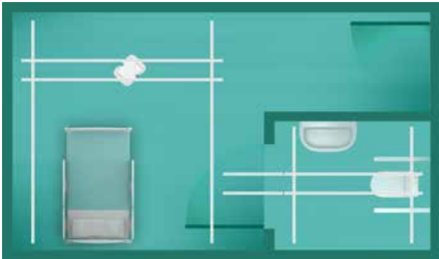
Two X-Y (Double Gate) solution Full-room coverage in both the patient's room and the en-suite, linked together with a straight track configuration using a Double Gate system.
