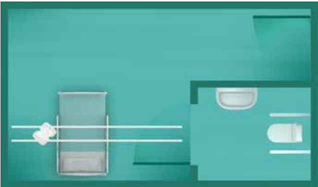
Straight track tracking solution A simple straight track configuration provides access for transfers on each side of the patient bed.
