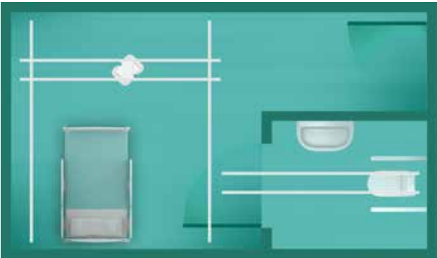
X-Y (single gate tracking solution) An X-Y tracking solution providing full room coverage within the patient's room combined with a Single Gate system and tracking leading into the en-suite bathroom.
