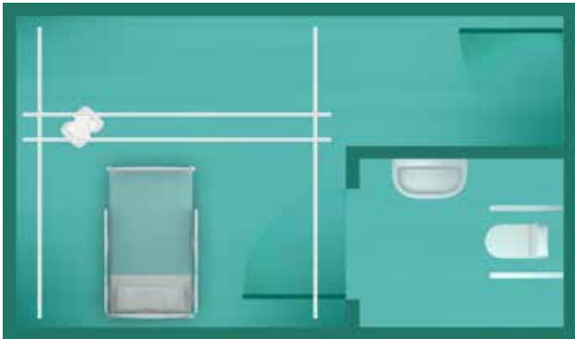
X-Y tracking solution An X-Y tracking solution provides full room coverage. A transfer can be performed anywhere within the two parallel tracks.
