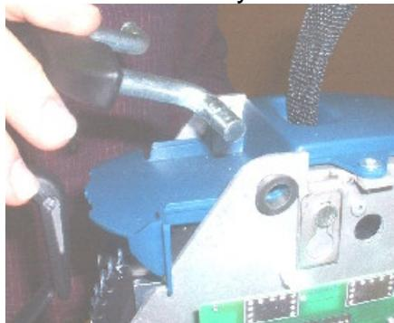
8. Insert the rings with the retaining ring pliers on each side of the handle. Be sure that the rings are in place and retain safely the handle.
