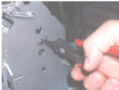
24. Remove the snap ring that maintains the strap roll shaft with the retaining ring pliers. Remove the shaft.
