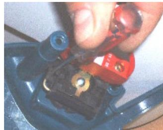
7. Remove both parts of the pushbutton to free the bottom and the main cabins.
