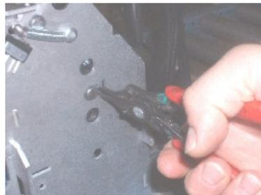
7. Reinsert the shaft then the strap roll on it. Be sure that the strap is behind the strap roll. Put the snap ring back with the retaining ring pliers.
