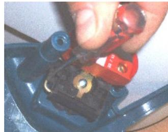
8. Remove both parts of the pushbutton to free the bottom and the main cabins.
