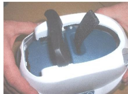
13. Fold completely the Tarzan hook. Make sure that the handle is inserted inside the cab.
