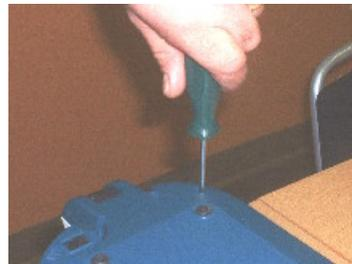
5. Slightly lift the cab to undercover the pushbutton.
