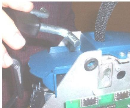
38. Insert the rings with the retaining ring pliers on each side of the handle. Be sure that the rings are in place and retain safely the handle.
