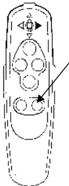
3. Press on the UP button to increase the lift capacity or on the DOWN button to decrease it. Each time you press the UP button, you add 5 lbs of lift capacity. Each time you press on the DOWN you reduce approximately 5 lbs of lift capacity. If you increase or reduce the lift capacity and that you hear 3 beeps instead of 1, you have reached the lift maximum adjustment.
