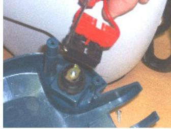
10. a) **To replace the button part**, simply unscrew from inside the cab. Remove the defective part and insert new button into the bottom cab. Screw the new button or
