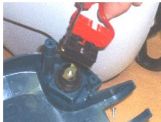
8. Unscrew the 2 tapping screws (item 2 on the exploded view) with a screwdriver Torx 20 to remove the battery support (item 34 on the exploded view).
