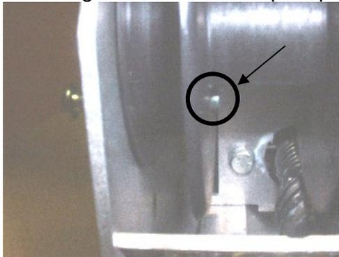
28. Keep the strap tight and screwing completely the lower screw into the loop with Allen key.
