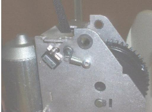
3. Drill the rivet out the rivet out from the other side and remove the upper limit shaft.
