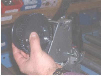
26. Remove the 3 screws that maintain the motor with a 12-mm socket.
