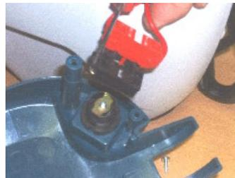
9. Unscrew the button part of the pushbutton and remove it.
