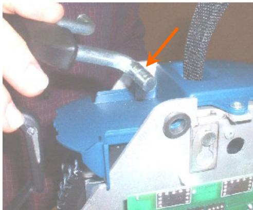
5. Insert the rings with the retaining ring pliers on each side of the handle. Be sure that the rings are in place and retain safely the handle.
