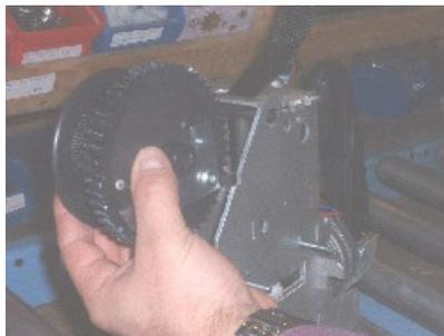
5. Insert the strap into the strap inlet. Insert the new drum into the frame then insert the shaft to maintain it.
