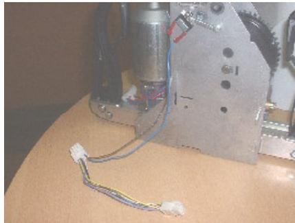
3. Replace wiring harness by a new one (Part number 402.16000)
