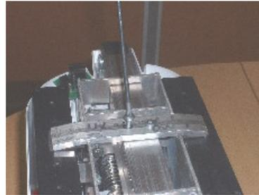
16. Put the button part of the pushbutton back, by inserting it from under the cab then screw it.
