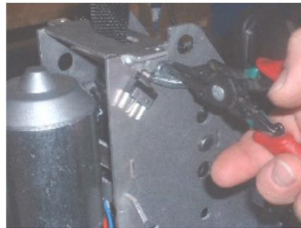
35. Plug the 2 wires back on both end of the limit switch. Never use the centre pin.
