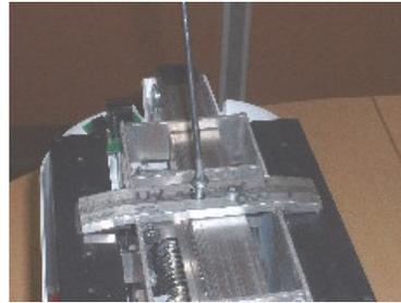
47. Put the button part of the pushbutton back, by inserting it from under the cab then screw it.
