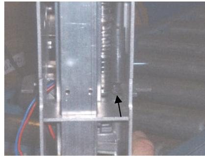
31. Put the drum back into the frame.
