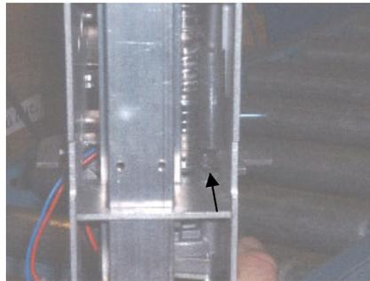
27. Remove the motor with the motor shaft from the frame and replace it by a new one.
