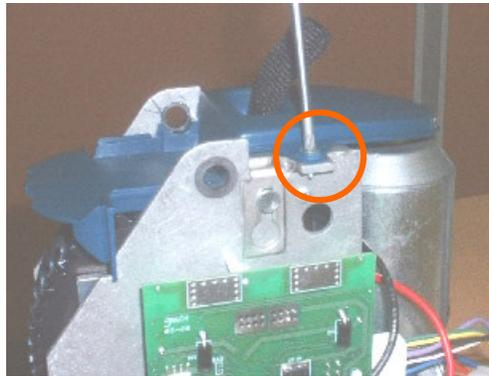
5. Replace with a new strap inlet (Item no 42 on the exploded view)
