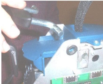
34. Insert the rings with the retaining ring pliers on each side of the handle. Be sure that the rings are in place and retain safely the handle.
