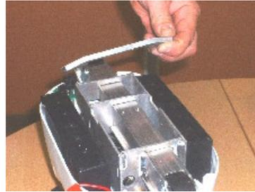
9. Remove the batteries and pull contact plugs.
