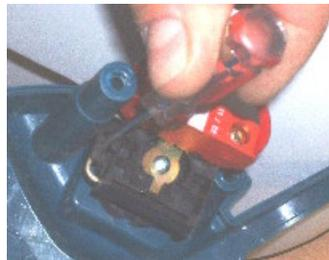
9. Remove both parts of the pushbutton to free the bottom and the main cabins.
