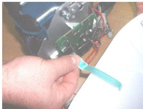
15. Remove the defective main and replace it by a new one.
