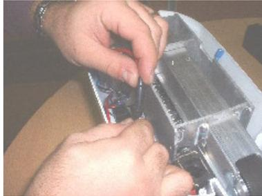
3. Remove the fuse and replace it by a new one (part number C8FGMA10).
