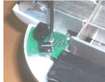
4. Replace the circuit by a new one.
