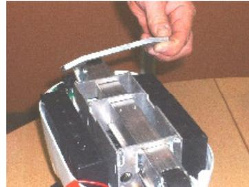
10. Remove the batteries and pull contact plugs.
