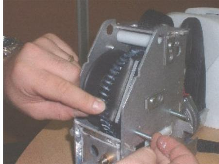
31. Plug the 2 wires back on both end of the limit switch. Never use the centre pin.
