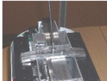
43. Put the button part of the pushbutton back, by inserting it from under the cab then screw it.
