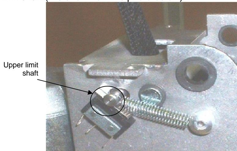
21. Plug the 2 wires back on both end of the limit switch. Never use the centre pin.
