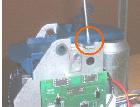
20. Unplug the 2 wires from the limit switch.
