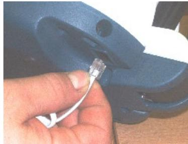
2. Replace it by a new hand controller and plug it to the lift.
