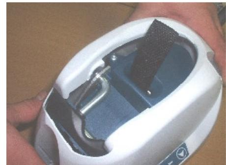
13. Slightly lift the main cab to free the touch pad membrane then unplug it from the main circuit board.
