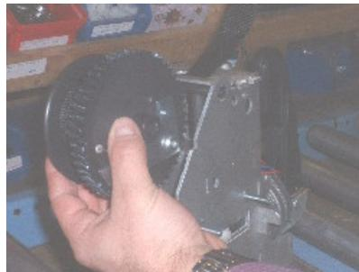
32. Insert the strap into the strap inlet. Insert the drum into the frame then insert the shaft to maintain it.
