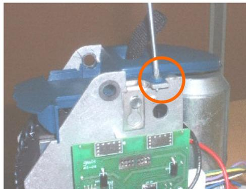
17. Unplug the 2 wires from the limit switch.
