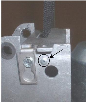
4. Insert the new upper shaft. Fix the rivet to maintain the upper shaft.
