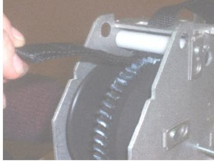
26. Align holes and insert manually the two button screws.
