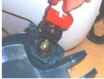
10. a) **To replace the button part**, simply unscrew from inside the cab. Remove the defective part and insert new button into the bottom cab. Screw the new button or
