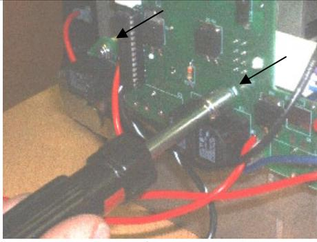
15. Unplug the charger/hand controller plug from the circuit.
