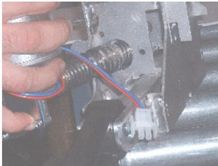
28. Insert the motor shaft into the frame. Couple the CBLM block plate into the slot at the end of the worm as shown below.
