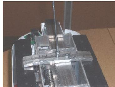
26. Put the button part of the pushbutton back, by inserting it from under the cab then screw it.
