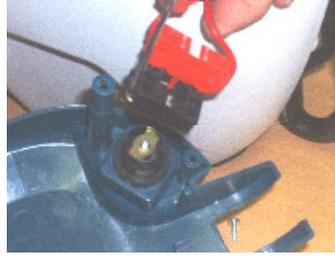
8. Unscrew the 2 tapping screws (item 2 on the exploded view) with a screwdriver Torx 20 to remove the battery support (item 34 on the exploded view).
