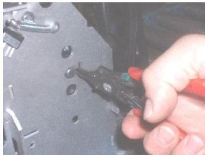
24. Remove the snap ring that maintains the strap roll shaft with the retaining ring pliers. Remove the shaft.
