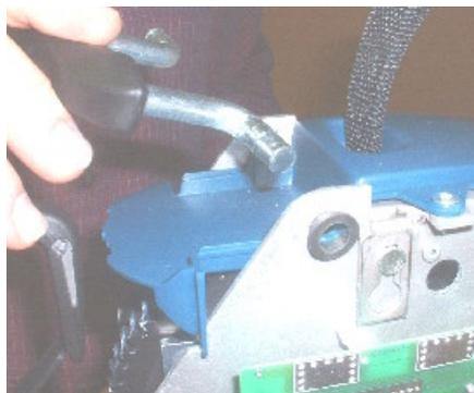
24. Insert the rings with the retaining ring pliers on each side of the handle. Be sure that the rings are in place and retain safely the handle.
