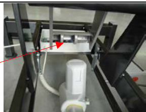
13. View after the shaft removal 7 (please note the spacers)
