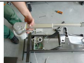
18. View of the removed actuator
