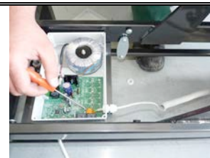
22. Connect actuator to controller using C
