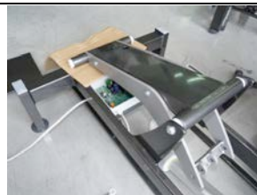
14. Position metal arms as shown and protect from damage
