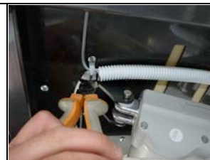
3* Cut the tie wrap 6 using B
