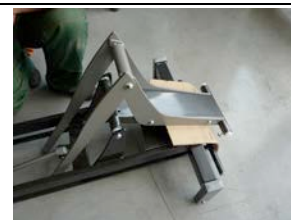
14. Position metal arms as shown and protect from damage
