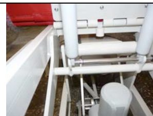
3a. Remove shaft item 8, please watch for plastic washers item 9
