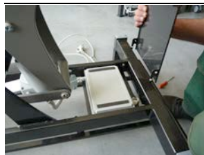
1. Remove the cover of the controller
