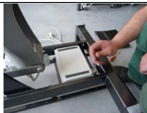
2. Remove the controller cover using E and remove the actuator's wires using C
