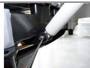
3. Remove E-Rings item 5 using tool C
