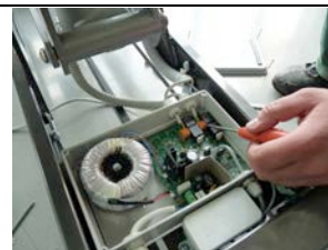
2. Remove the controller cover using E and remove the actuator's wires using C
