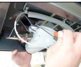
2. Remove E-Rings item 3 using C
