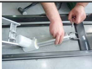
19. Start installing new actuator by first inserting shaft item. 5
