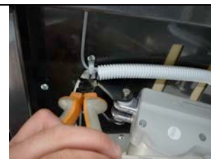
3. Cut the tie wrap item 6 using B
