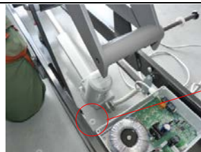
13. View after the shaft removal 7 (please note the spacers)
