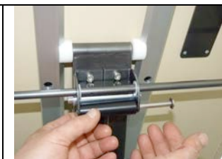
1. Remove cap item. 6 and E-ring item 8 using A and remove piston item. 5
