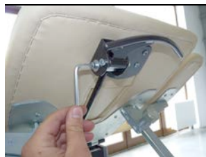
1. Un-tighten screws item 7 using tool B
