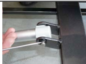
16. Remove E-Rings item 4 using C
